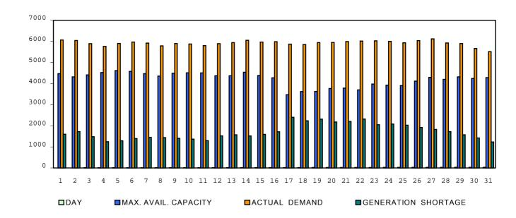
INSTALLED CAPACITY = 8090 MW
